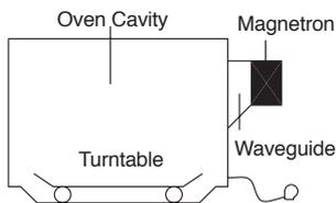
In a microwave oven, electricity is converted into microwave by the **MAGNETRON**.
