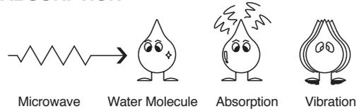
The microwaves cause the water molecules to vibrate which causes **FRICTION**, i.e. **HEAT**. This heat then cooks the food. Microwaves are also attracted to fat and sugar particles, and foods high in these will cook more quickly.
